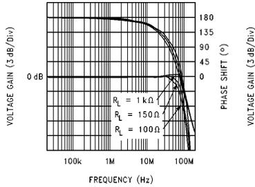
**Inverting Gain Frequency Response**
