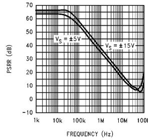
**PSRR ( $V_{S-}$ ) vs Frequency,  $A_V = 2,$
