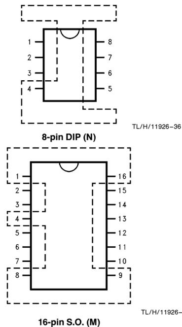
**FIGURE 11. Copper Heatsink Layouts**
