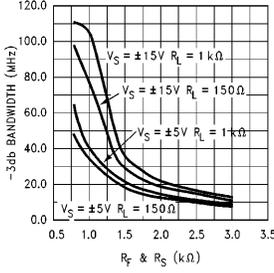
**Inverting Gain vs -3 dB Bandwidth**
