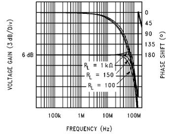
**Non-Inverting Gain Frequency Response**
