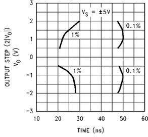
**Settling Time vs Output Step,  $R_F = 820\Omega$ ,  $R_L = 150\Omega$ ,  $A_V = -1$**
