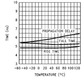
**Small Signal Pulse Response vs Temperature, AV = +2, VS = ±15V, RL = 1kΩ**
