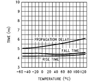
**Small Signal Pulse Response vs Temperature, AV = -1, VS = ±15V, RL = 150Ω**
