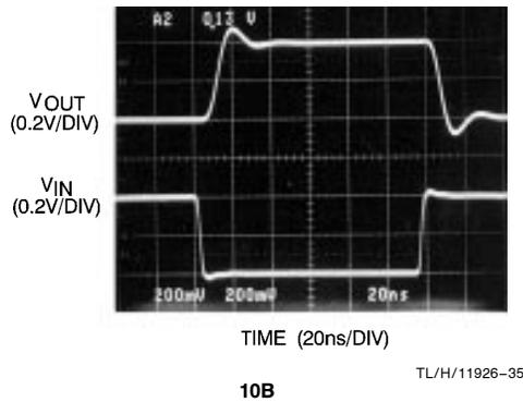
**FIGURE 10A, 10B. Resistive Isolation of  $C_f$  Provides Higher Fidelity Pulse Response.  $R_f$  and  $R_s$  Could Also Be Increased to Maintain  $A_V = -1$  and Improve Pulse Response Characteristics.**
