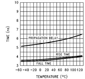
**Small Signal Pulse Response vs Temperature, AV = +2, VS = ±15V, RL = 150Ω**
